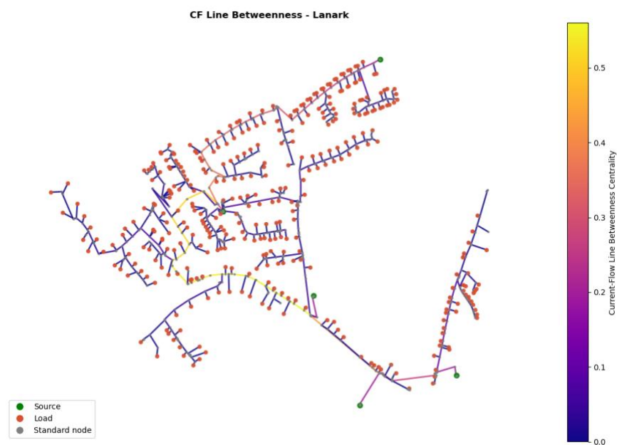
Figure 43: Visualization of current-flow line betweenness centrality values in the Lanark network
