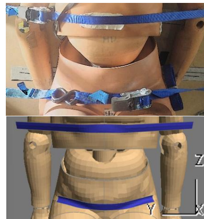
1 Fig. 1. H3 initial position in experimental testing (top) 4 Fig. 2. Restraining heavy-duty cargo strap position for 2 and in FE environment (bottom) 5 torso and pelvis in experimental testing (top) and in 3 6 FE environment (bottom)
