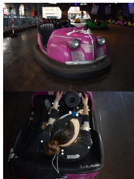
Figure 1a-b: (top) Bumper-car vehicle set-up with VICON markers attached to vehicle and on-board GoPro camera. (bottom) Example test of volunteer rotating head approximately 45° to the right for a rear-end impact.
