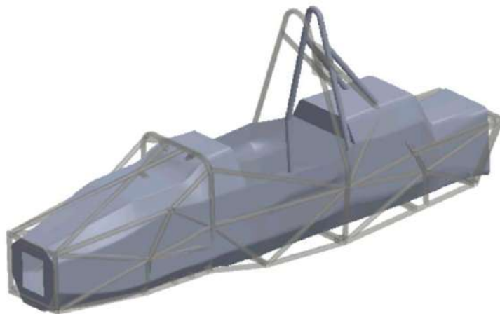
Figure 5. Overlay of a tubular steel frame and the monocoque.
