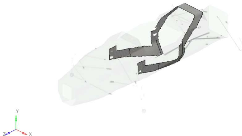
Figure 105 Hoop set isometric view
