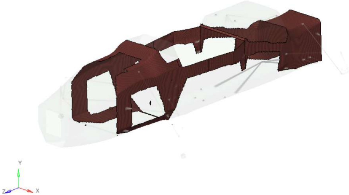
Figure 43 Final suspension plies set
