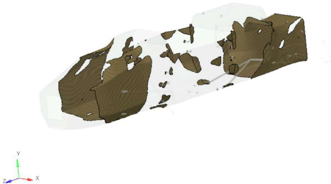
Figure 41 Free sizing example with suspension loads
