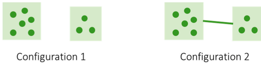
Fig. 4. The two configurations considered. Configuration 1 includes two clusters that are electrified separately, whereas configuration 2 considers that both clusters are electrified together. The green dots represent consumers, and the green segment represents a distribution line connecting the two clusters.
