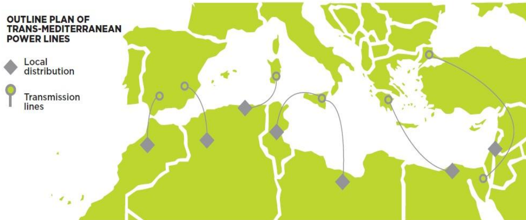
Figure 4: Electrical interconnections expected by the project MEDGRID.
