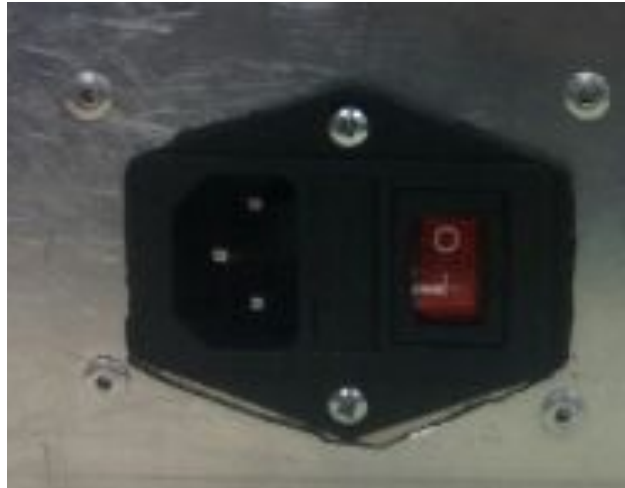
Figure 18- Power Socket with Switch
