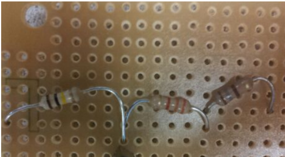
Figure 21- Visual Of Step Down Resistor
