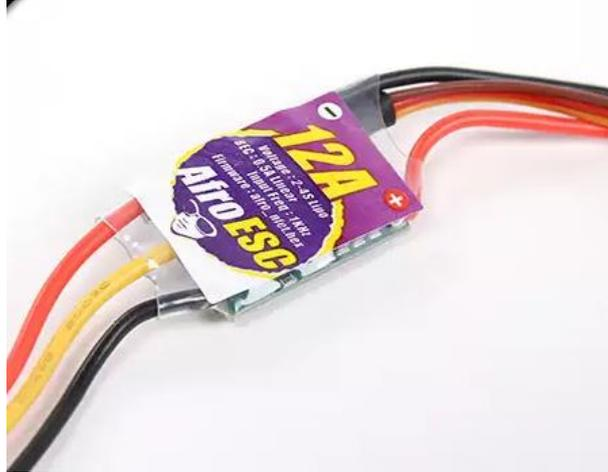
Figura 2.5 Afro ESC 12Amp BEC UltraLite
