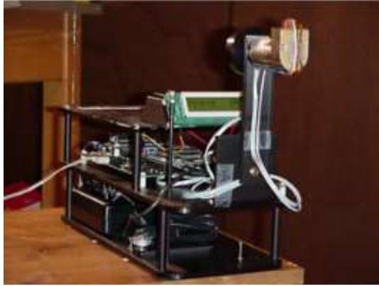
Figura 3: Reaction Wheel Pendulum
