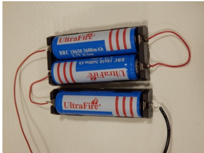
Figure 19. Batteries connected in series
