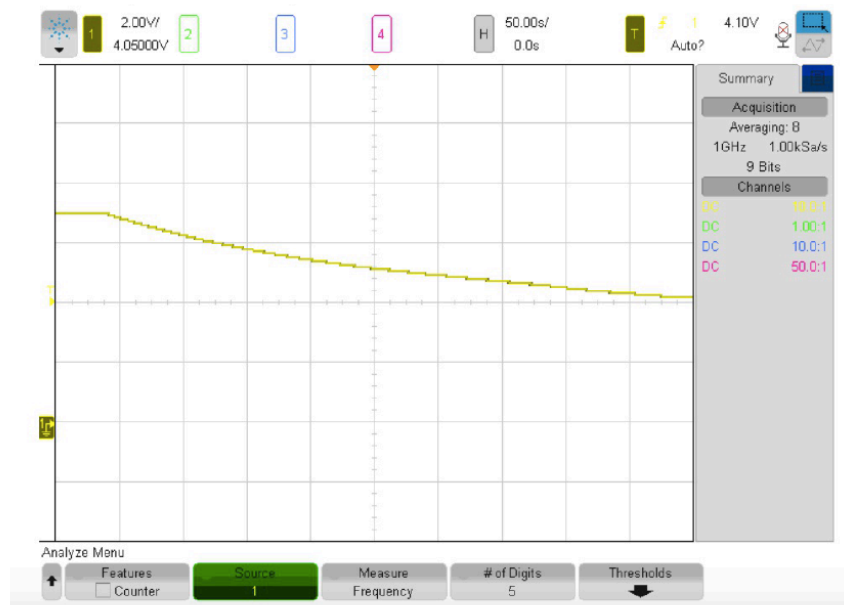
Figure 26. Capacitor discharge rate.
