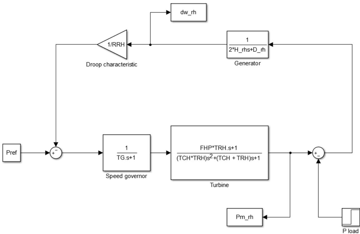
Figure 13: Block diagram of the reheat unit [5].
