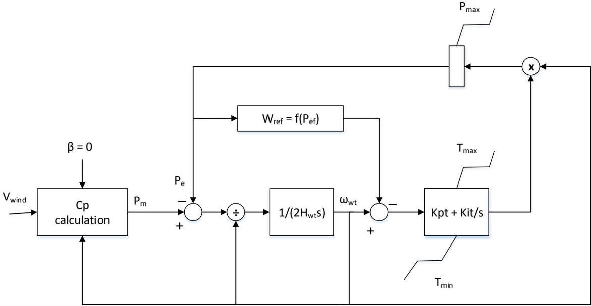
Figure 9: Block diagram of VSWT [18], [8]
