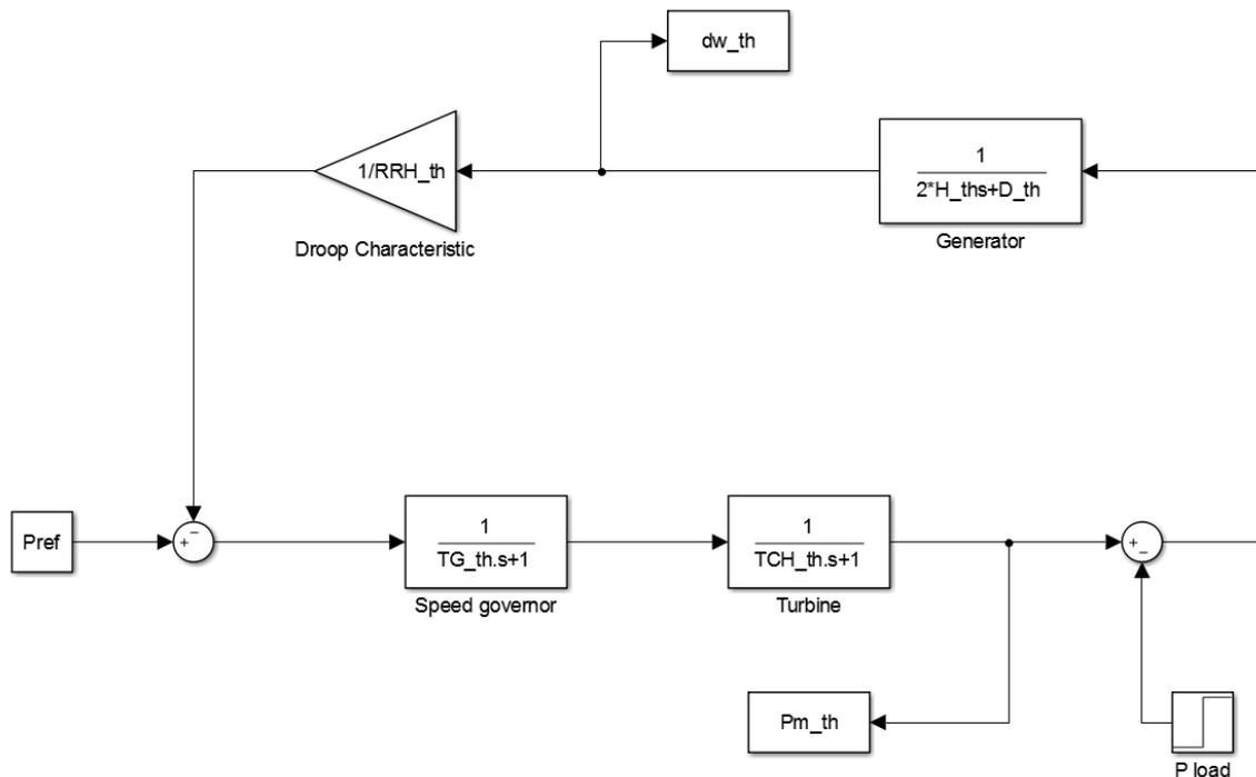
Figure 12: Block diagram for the thermal unit [5].
