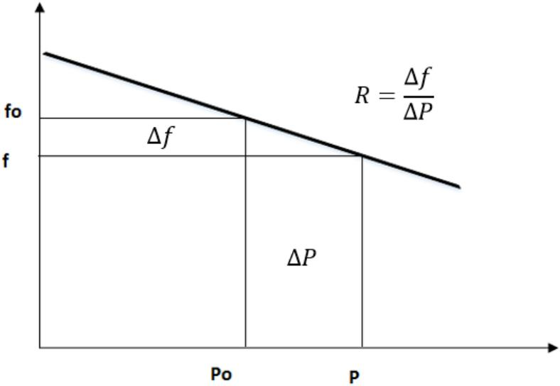
Figure 1: Ideal steady-state characteristic of a speed-droop governor [5].
