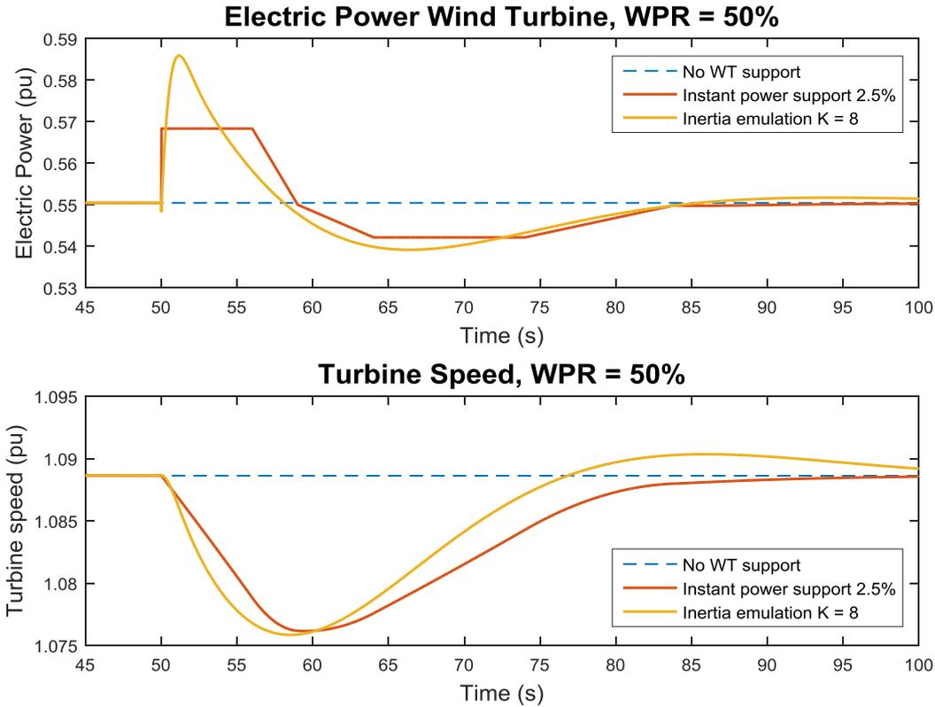
Figure 23: Deceleration and re-acceleration areas and rotor speed. Hydro and reheat units operating, WPR = 50%
