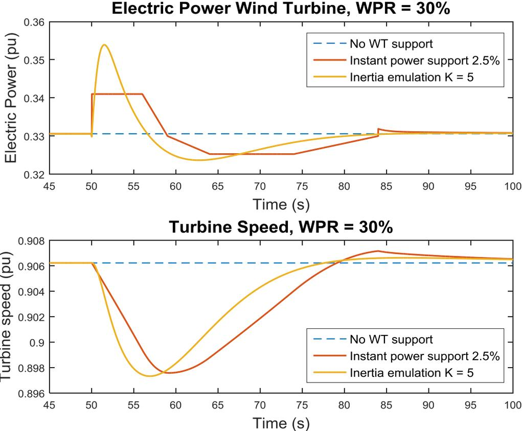
Figure 19: Deceleration and re-acceleration areas and rotor speed. Hydro and reheat units operating, WPR = 30%
