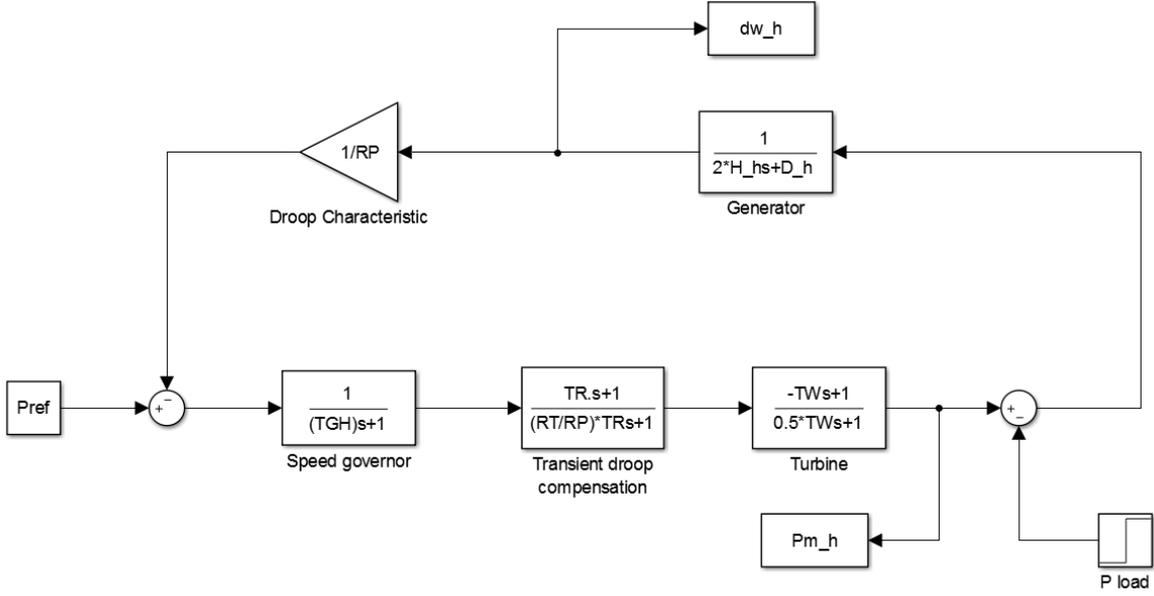
Figure 11: Block diagram for the hydro unit [5].
