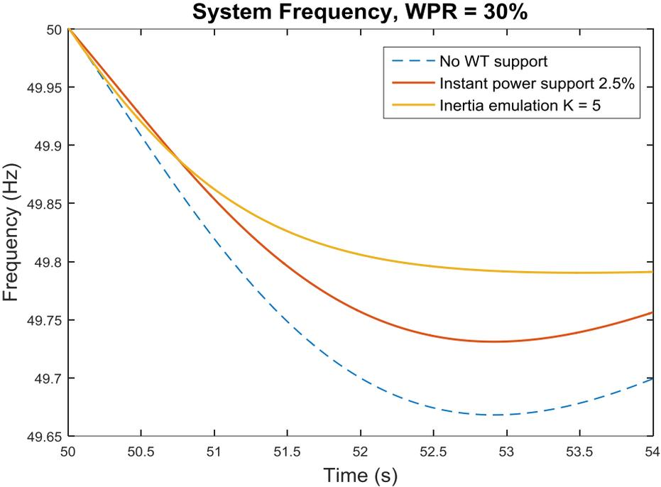
Figure 18: Enhanced view of nadir for different strategies. Hydro and reheat units operating, WPR = 30%
