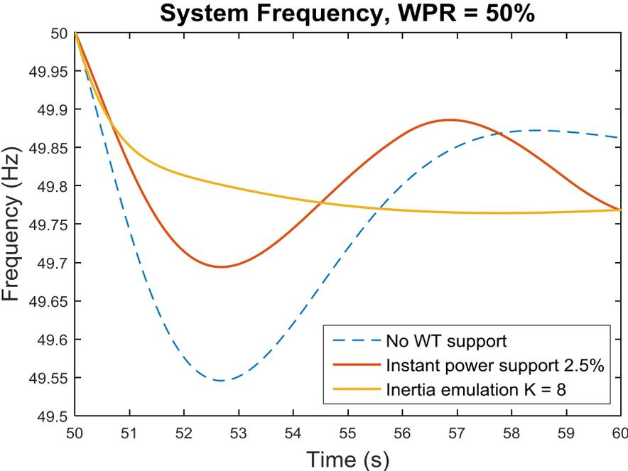
Figure 22: Enhanced view of nadir for different strategies. Hydro and reheat units operating, WPR = 50%
