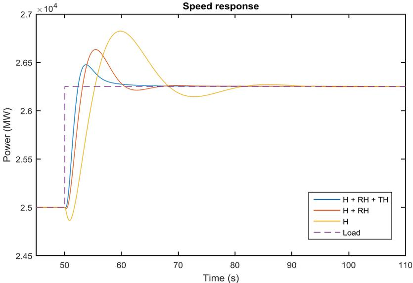
Figure 16: Droop response of different combination of responding units to a load step of 5%
