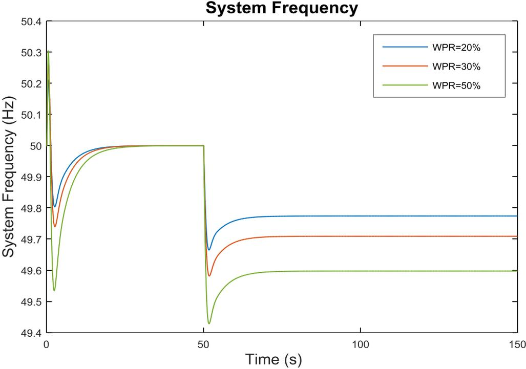
Figure 5: Frequency response to power step for different values of WPR
