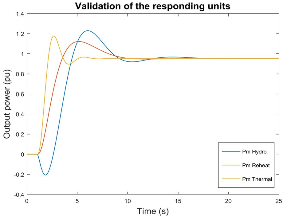
Figure 14: Power response of responding units to a sudden increase in the load
