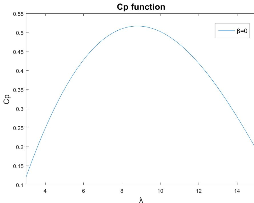
Figure 8: Power coefficient for different values of  $\lambda$  and  $\beta = 0$
