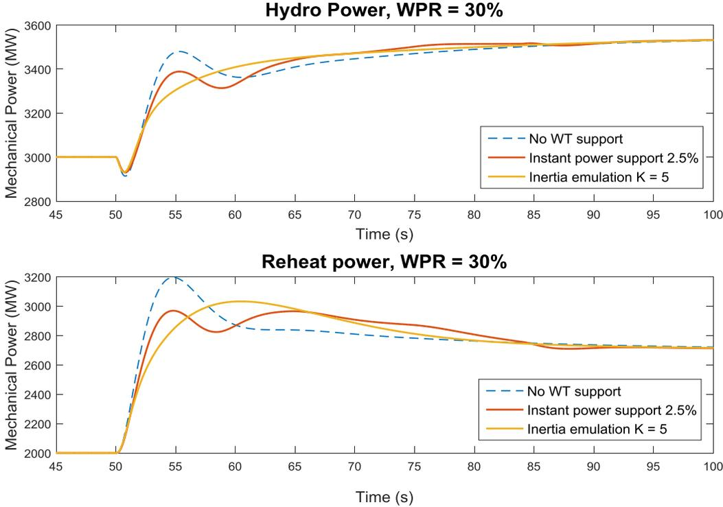
Figure 20: Droop response of hydro and reheat units, WPR = 30%
