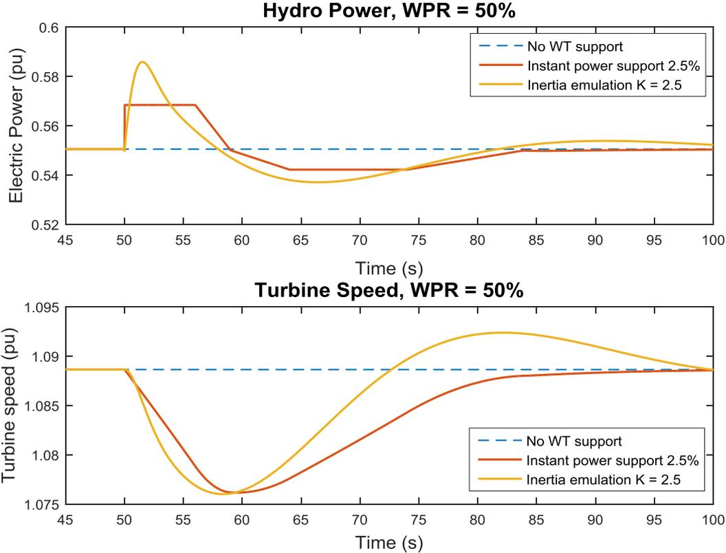
Figure 31: Deceleration and re-acceleration areas and rotor speed. Hydro unit operating, WPR = 50%
