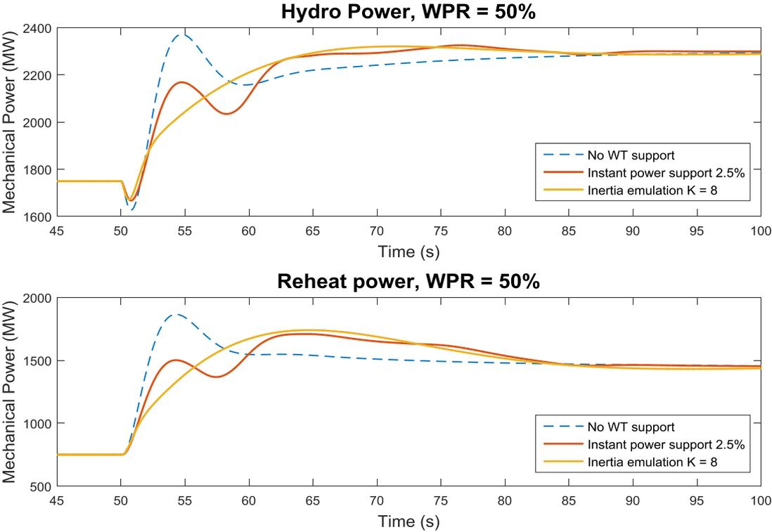
Figure 24: Droop response of hydro and reheat units, WPR = 50%
