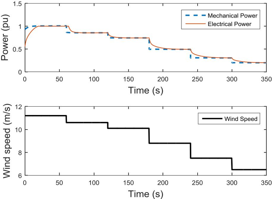
Figure 10: Power response of WT for different wind speeds
