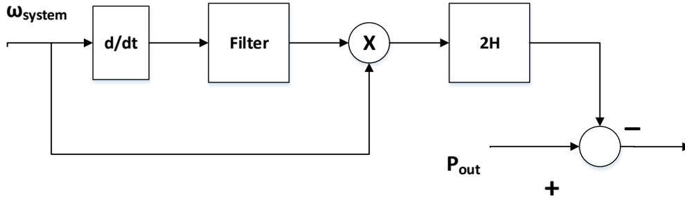
Figure 4: Inertia emulation support block diagram [7]
