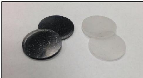
Figure 3 - 19: Discs of KBr with and without powder nanomaterial for the measurement of the FTIR spectra
