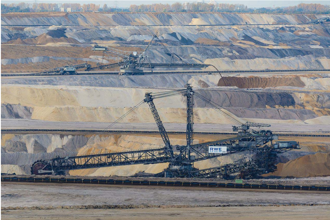
Figure 3.27: Bucket-wheel excavators mining brown coal at the Inden opencast mine, Germany. Image from Wikimedia Commons. Photo by CEphoto, Uwe Aranas [CEp]
