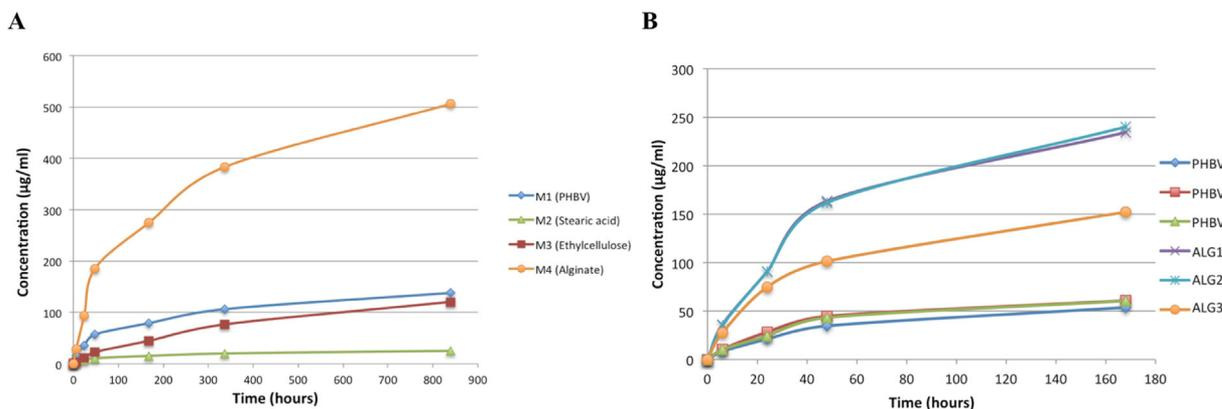
**Figure 3.** (A) Cumulative rifampicin elution from PHBV, stearic acid, ethylcellulose and alginate microcapsules over 5 weeks. (B) Cumulative rifampicin elution from PHBV and alginate microcapsules over 1 week.
