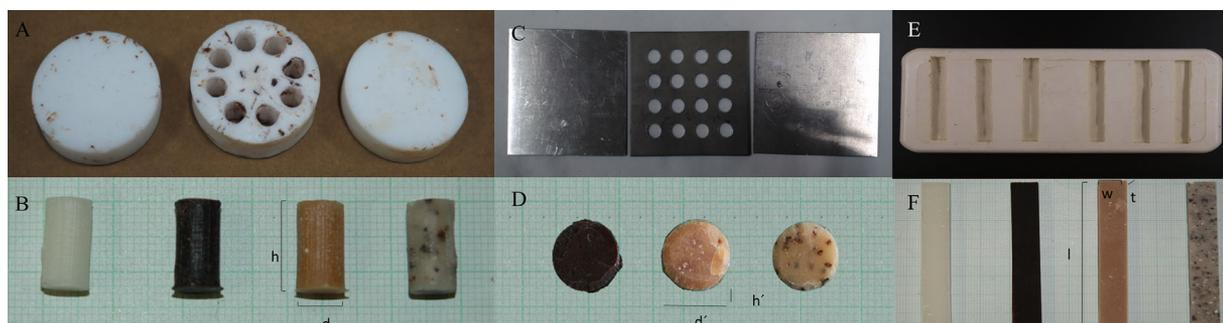
**Figure 2.** Molds and bone cement samples. (A and B) Elution and compression tests (h: height, d: diameter). (C and D) Microbiological tests (h': height, d': diameter). (E and F) Flexion tests (l: length, w: width, t: thickness).
