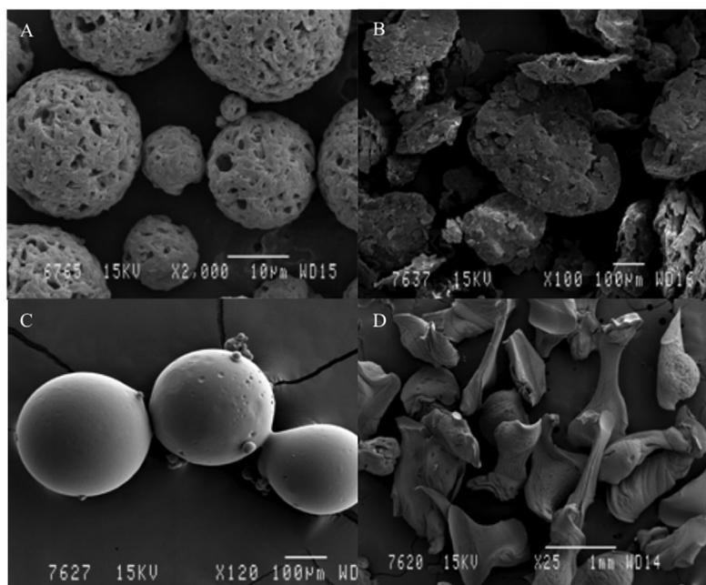
**Figure 1.** SEM images of the microcapsules. (A) PHBV. (B) Stearic acid. (C) Ethylcellulose. (D) Alginate.
