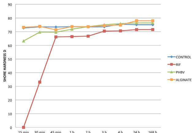
**Figure 5.** Hardness behavior over time (Shore D scale).
