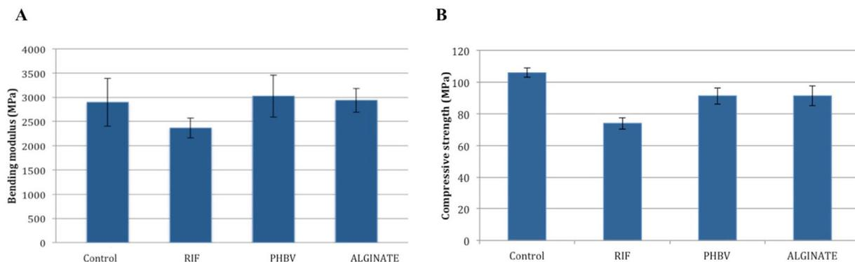
**Figure 4.** (A) Bending modulus of the bone cement samples. (B) Compressive strength of the bone cement samples.
