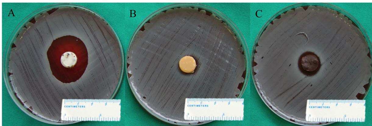
**Figure 7.** Zones of inhibition produced by bone cement with alginate microcapsules (A), PHBV microcapsules (B) and rifampicin (C) Powder Phase.
