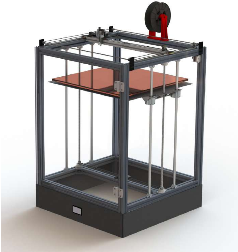
Figure 15: First design CAD File Frame with gantry, bed, and enclosure
