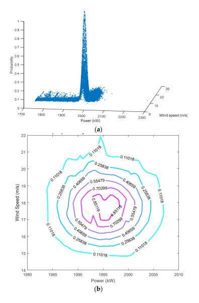
**Figure 3.** Probability distribution function for the pattern representing the highest production of electricity in the wind turbine: (**a**) tridimensional scatter plot; (**b**) probability contour plot.
