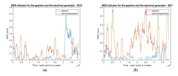
**Figure 9.** Non-expected behavior (NEB) indicators for the gearbox and the electrical generator in the years 2010 (**a**) and 2011 (**b**).
