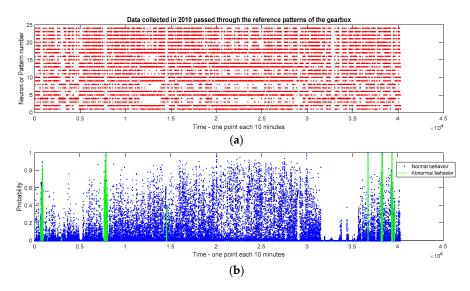
**Figure 7.** Data collected in 2010 and passed through the 24 patterns discovered characterizing the behavior of the gearbox of the wind turbine in 2009: (a) The graph presents the neuron representing the sample; (b) the graph shows the probability that the sample belongs to the associated pattern. The anomalies detected are in green indicating a probability of being an anomaly.
