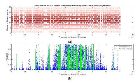
**Figure 8.** Data collected in 2010 and passed through the 24 patterns discovered characterizing the behavior of the electrical generator of the wind turbine in 2009: (**a**) The graph presents the neuron representing the sample; (**b**) the graph shows the probability that the sample belongs to the associated pattern. The anomalies detected are in green indicating a probability of being an anomaly.
