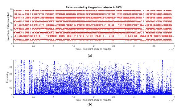
**Figure 5.** Training set data passed through the 24 patterns discovered characterizing the behavior of the gearbox of the wind turbine: (**a**) The graph presents to the neuron representing the sample; (**b**) the graph shows the probability belonging to the associated pattern.
