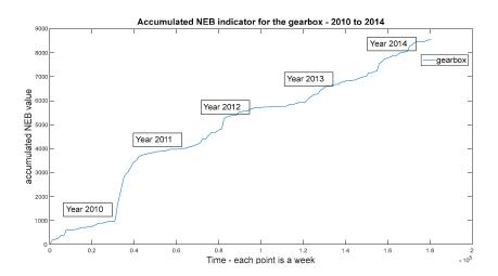
Figure 10. Accumulated NEB indicator for the gearbox between 2010 and 2014.
