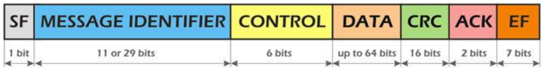
Illustration 2 - CAN Protocol overhead scheme [6]
