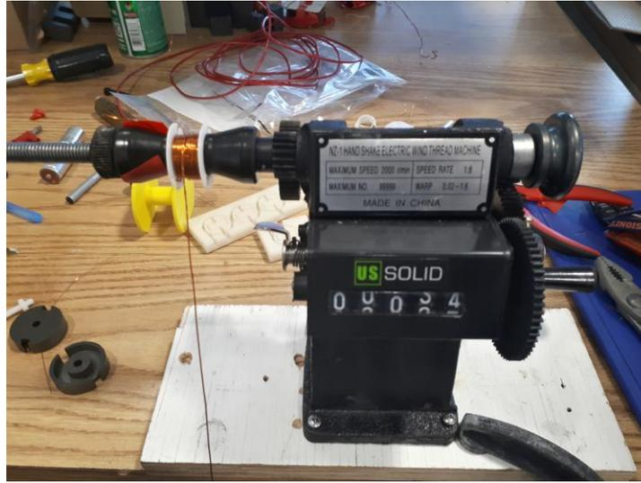
**Figure 4.1.** Process of winding a coil for the inductor  $L_2$ .
