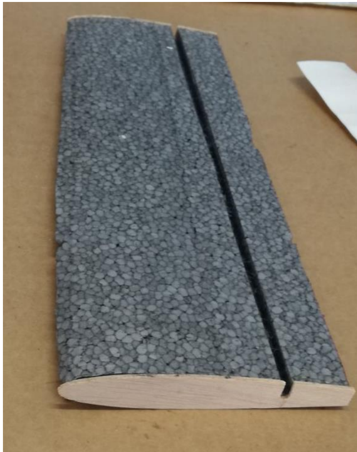
Figure 26: Horizontal stabilizer with foam cut.
