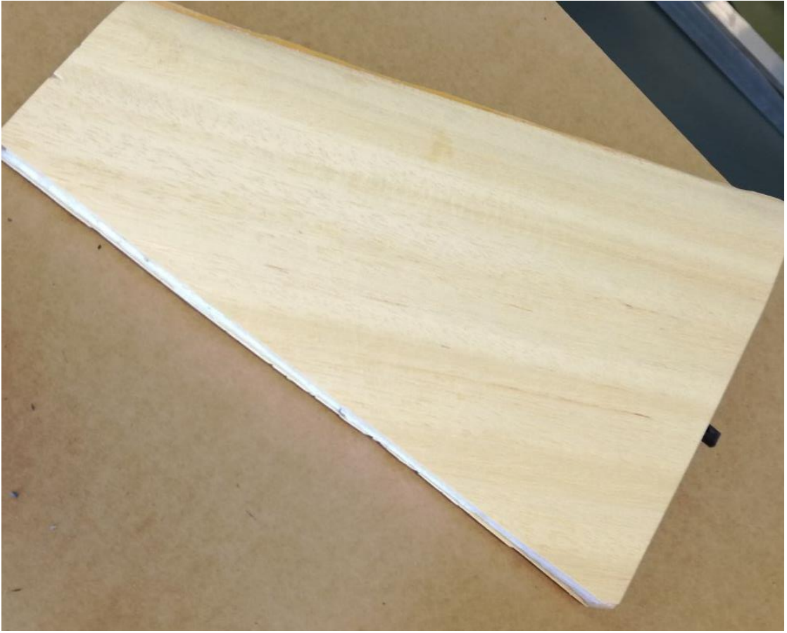
Figure 49: Vertical stabilizer covered out of wood.
