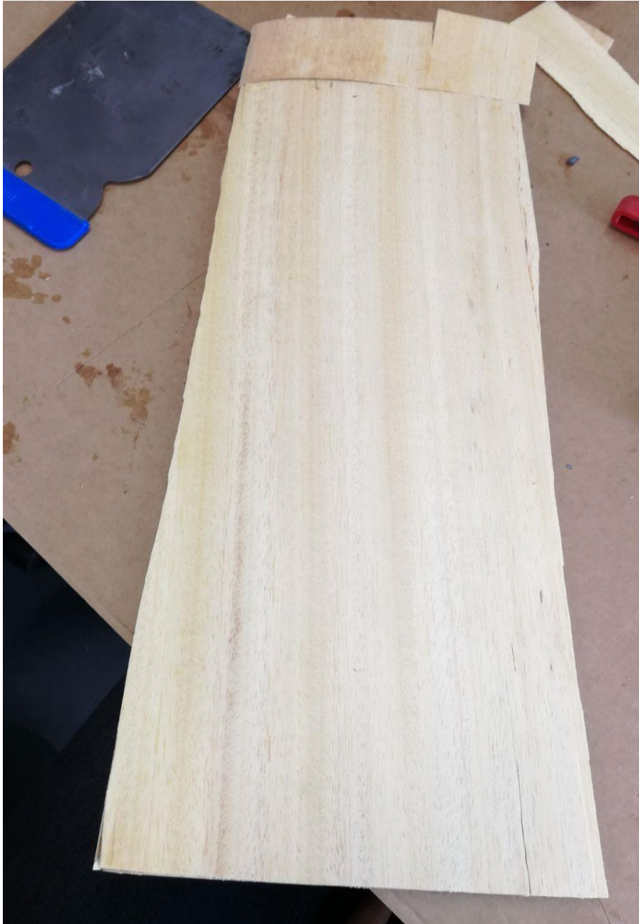
Figure 29: Part of the horizontal stabilizer covered out of wood
