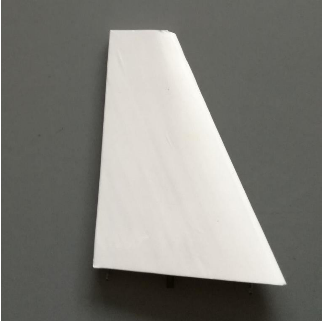
Figure 54: Vertical stabilizer covered out of plastic.
