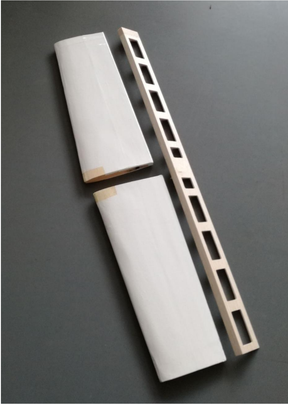
Figure 36: How the finished parts of the horizontal stabilizer would fix.
