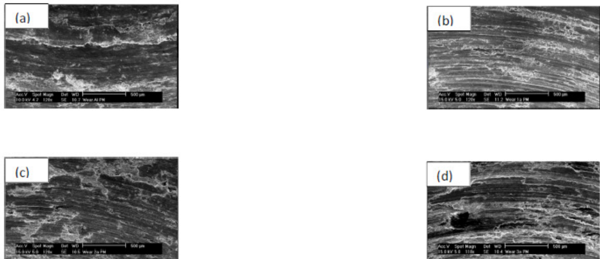
Figure 5 SEM images for tracing the elements present in Powder Metallurgy Specimens;Zoom level=100μm; Dark Grey=Al 2 O 3 ;Light Grey=Al; Black between grains=Al/C/Mg/O;Bright and White Points=ZnO/Fe 2 O 3 (on the Surface);Bright and White Points=MgO(embedded);
