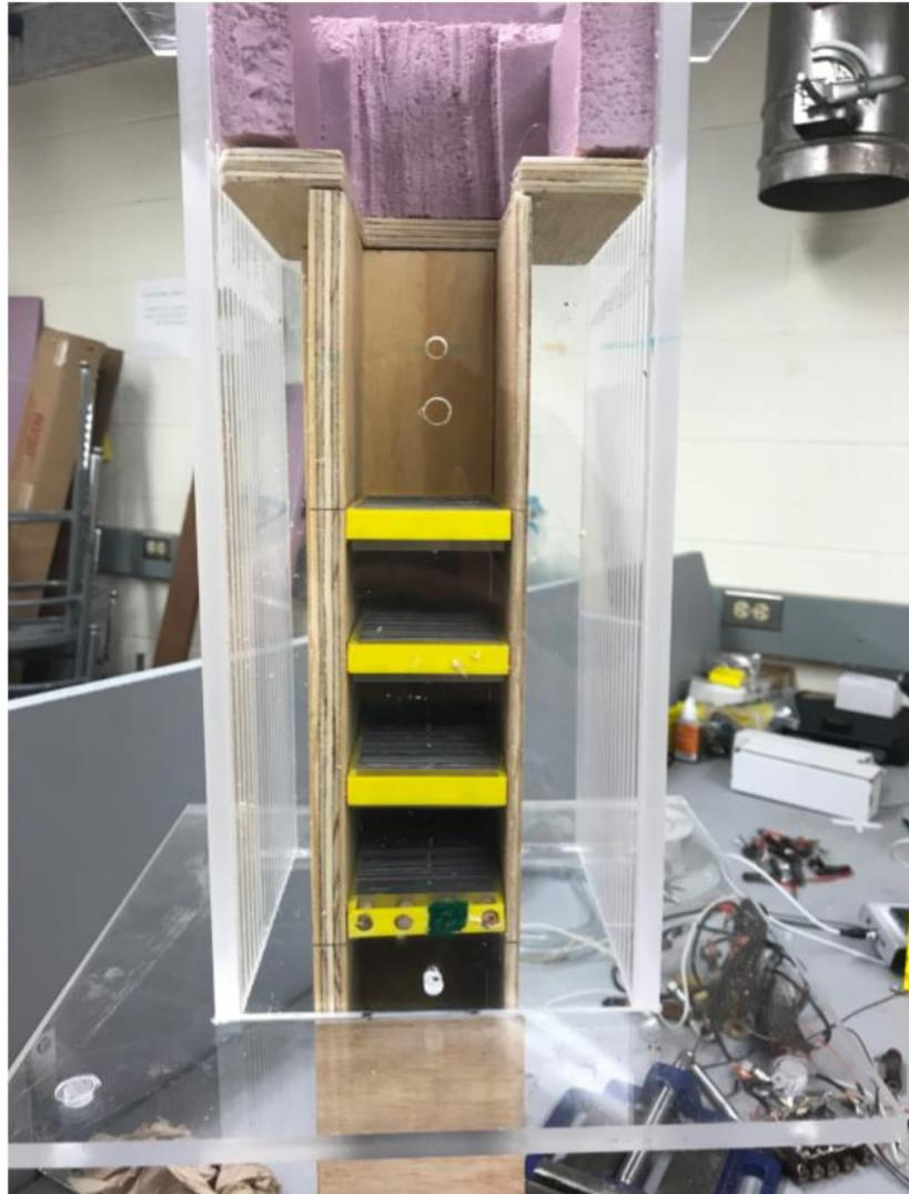
*Figure 32: Pressure Drop Experiment Setup*
