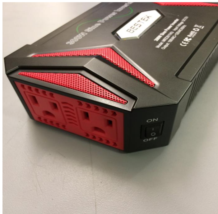
Figure 47. Switch on DC-AC inverter for discharge station.
