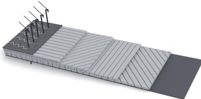
.Non-crimp fabrics behave as a laminate composed by various plies of unidirectional fabrics, stacked following a specific sequence and orientation. Therefore, NCF mechanical properties can be obtain applying directly CLT. It is assumed that the amount of stitching material compared to the lamina weight is negligible, and for that reason it does not influence on the stack properties.
