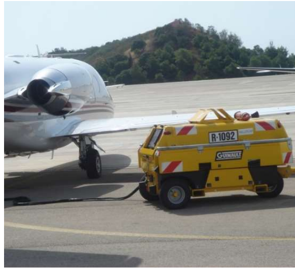
(fig. 2): Ground Power Unit [4]
