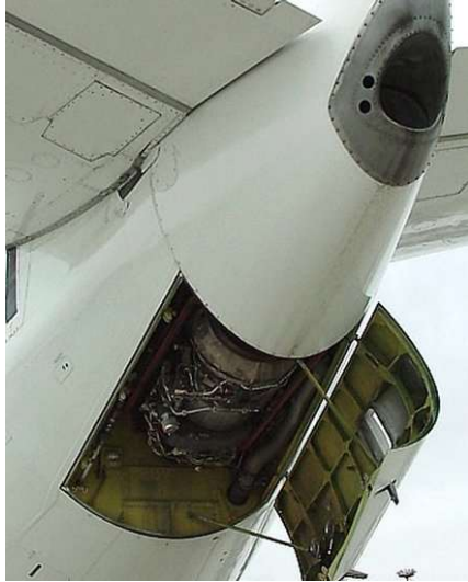
(fig. 1): Auxiliar Power Unit [4]
