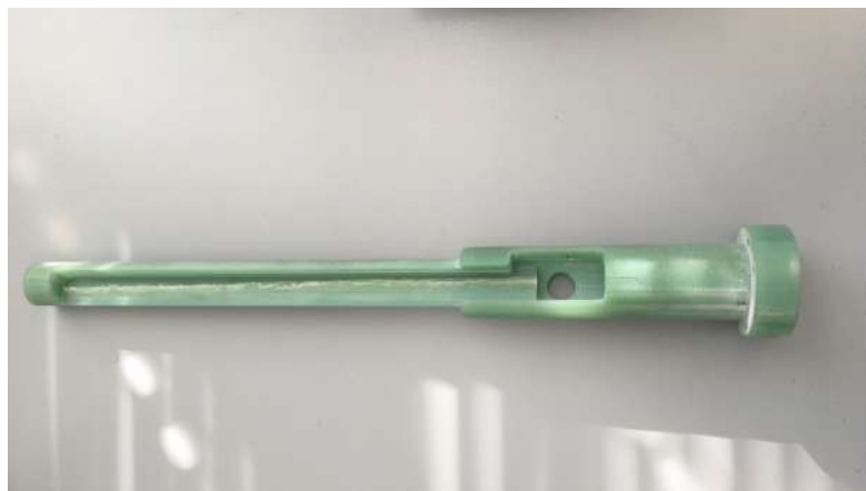
Figure 42: Mole used to couple the PCB to the rotation stage
