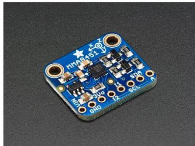
*Figure 85: Accelerometer [10]*
