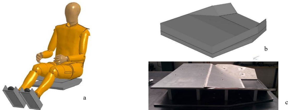
Fig. 2. Seat modification a) THOR in SAFER seat, b) FE seat model, c) seat hardware
