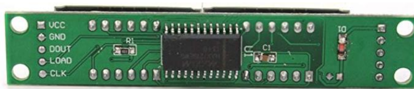
Figure 20: MAX7219 display pin connections. Source: Banggood, 2019 [15]
