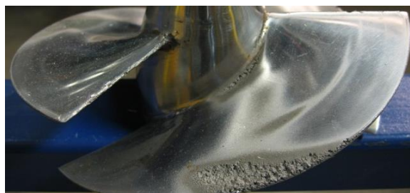
Figure 7. Effects of Cavitation on the Blades of a Turbine
