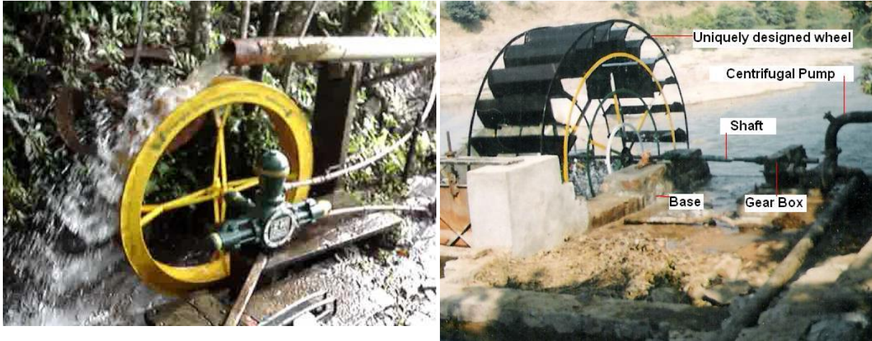
Figure 40. ZM 51 pump by ZM Bombas; Mangal Turbine
