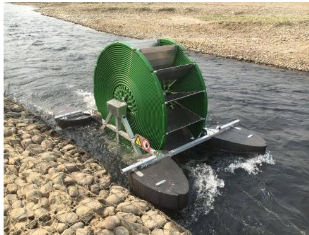
Figure 1. Barsha Pump operating
