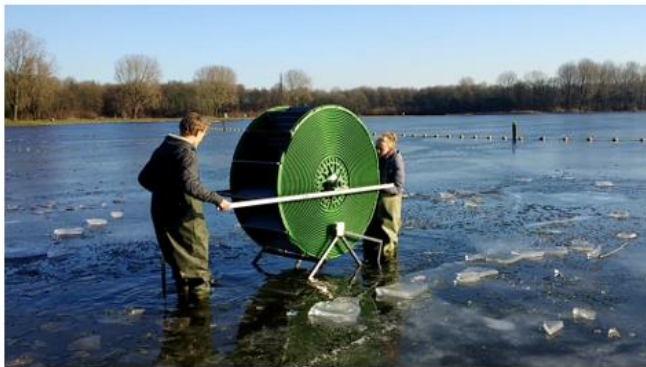
Figure 43. On the left, hydropowered pumping system with handles; on the right, a pump in a wheeled structure
