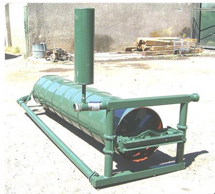
Figure 39. Hydrobine by EB Engineering; Ndume Turbo water pump
