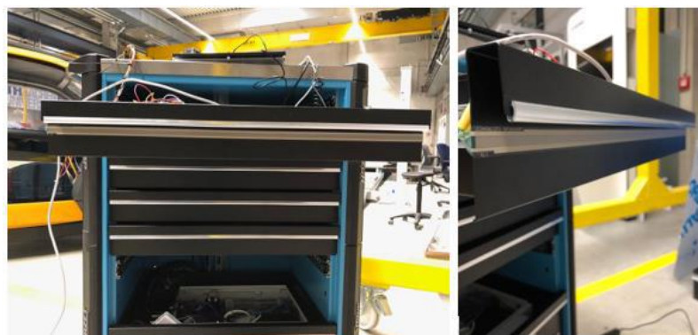
Figure 5: Force resistive sensor on the front part of the drawer
