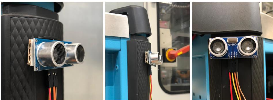
Fig. 4.8: Ultrasonic sensors on the trolley
