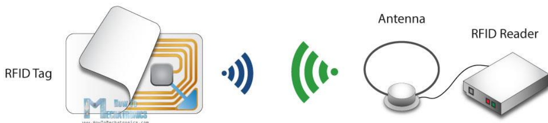
Fig. 3.9: Components of an RFID system (12)
