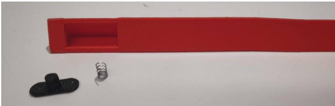
Figure 33: Outer piece, lateral view, with the spring and the button
