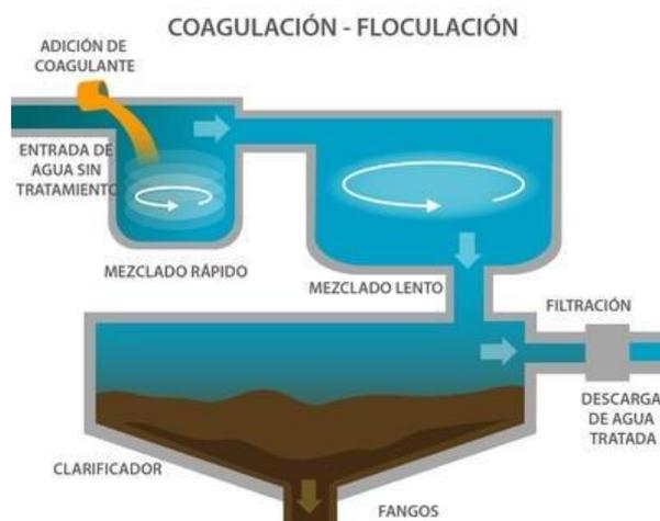
Figure 3: graphic representation of the basic treatment
