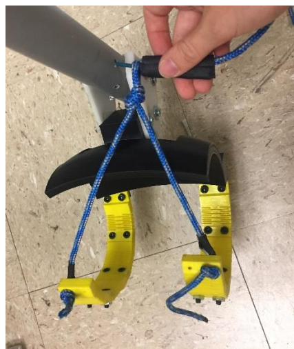
Figure 42. Pin release using ropes
