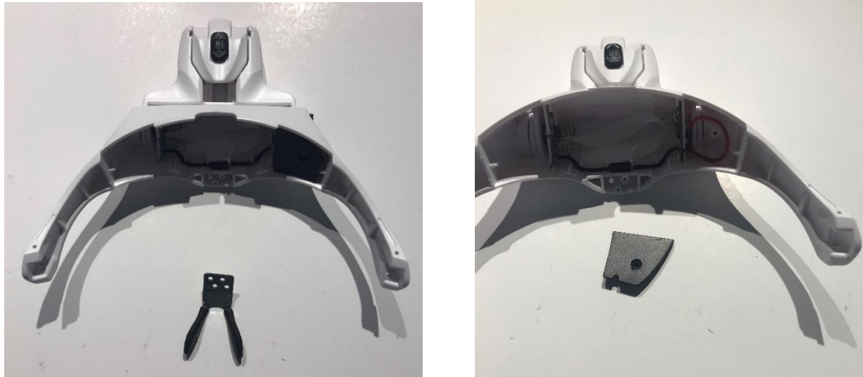
Figure 6: Disassembling of the nose adjuster and disassembling of the inside top
