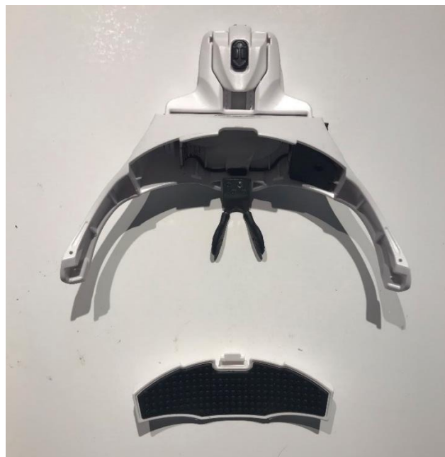
Figure 5: Disassembling of the rubber front pad
