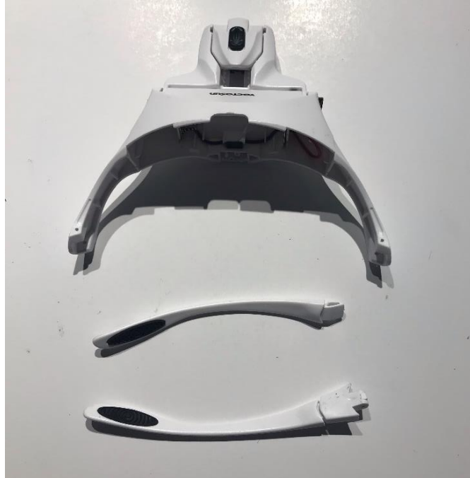
Figure 4: Disassembling of the ear temples
