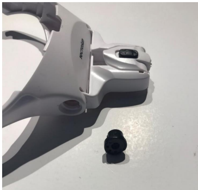
Figure 7: Disassembling of one of the cylindrical side plugs
