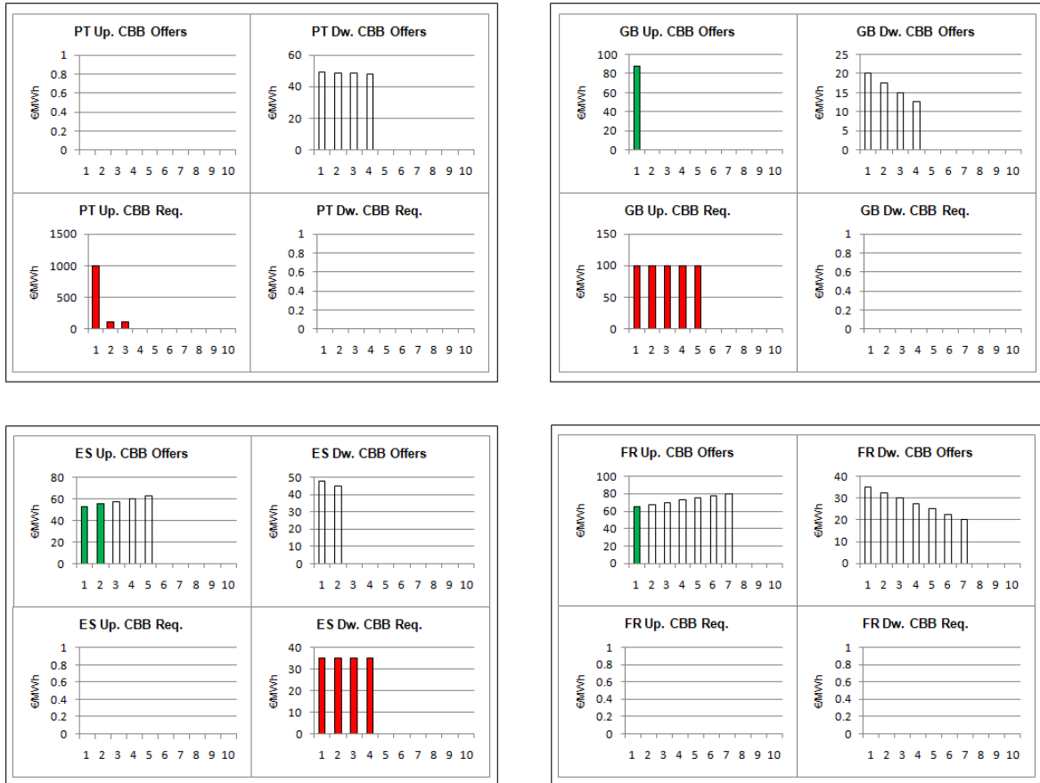
Figure 5.36 – Activated (solid) and not activated (hollow) tenders (surpluses in the first part of the bidding curve) †
