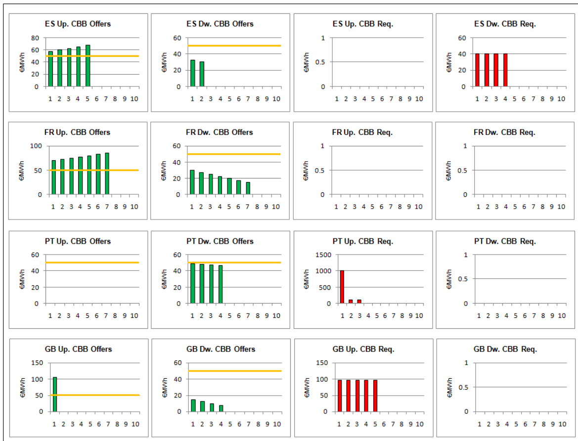
Figure 5.40 – Offers (green) and requirements (red) sent to the cross border balancing platform, and reference price (orange) (surpluses in the last part of the bidding curve) †
