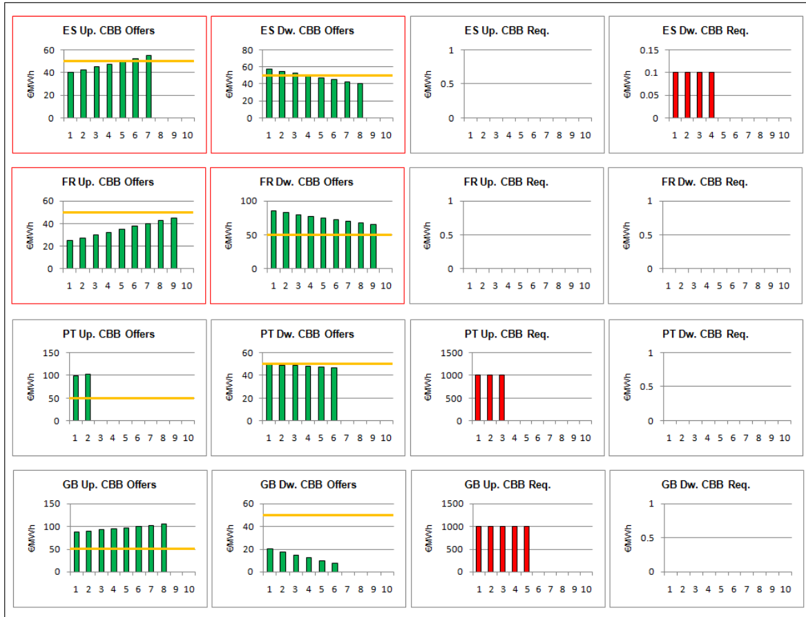
Figure 5.12 – Offers (green) not considering the reference price (orange) rule in Spain and France (red frames) †
