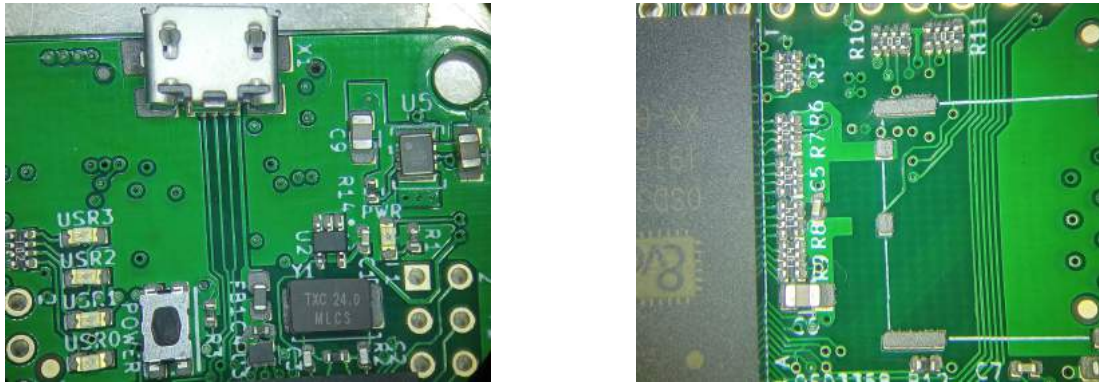
Figure 5.15: Components placed onto their footprints with the solder paste.
