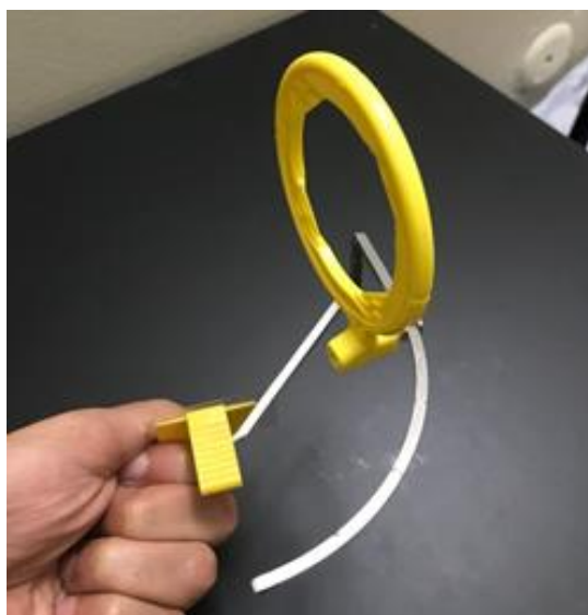
Figure 24. Device proposed by the customer, where a new bar that allows rotating the ring and the x-ray cannon is used.
