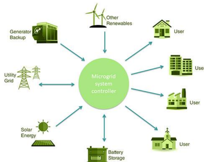
Figure 2.1 microgrid General Scheme [4]
