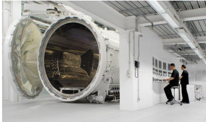
Figure 58 – Autoclave used in F1 competition to manufacture carbon fiber parts
