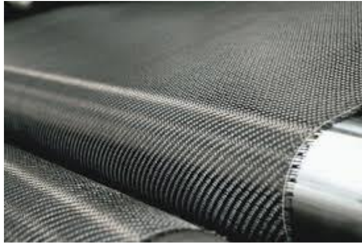
Figure 56 – Carbon fiber sheet after surface treatment
