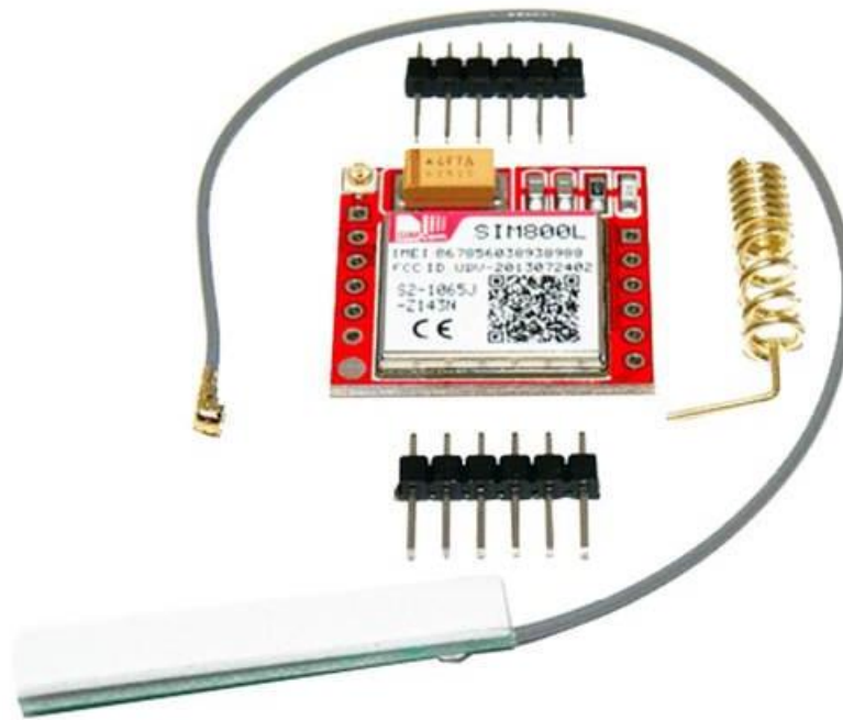
Figure 17. SIM800L module used in the second prototype [42].
