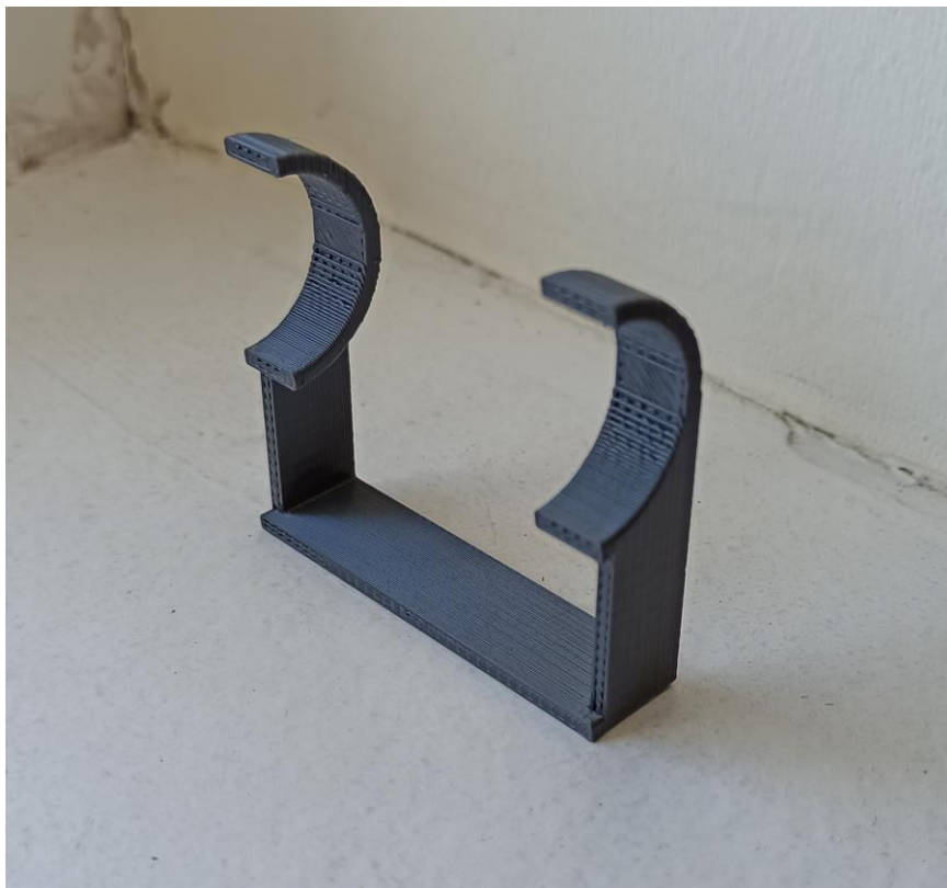
Figure 42. Half of the 3D printed frame for the cylindrical flow meter
