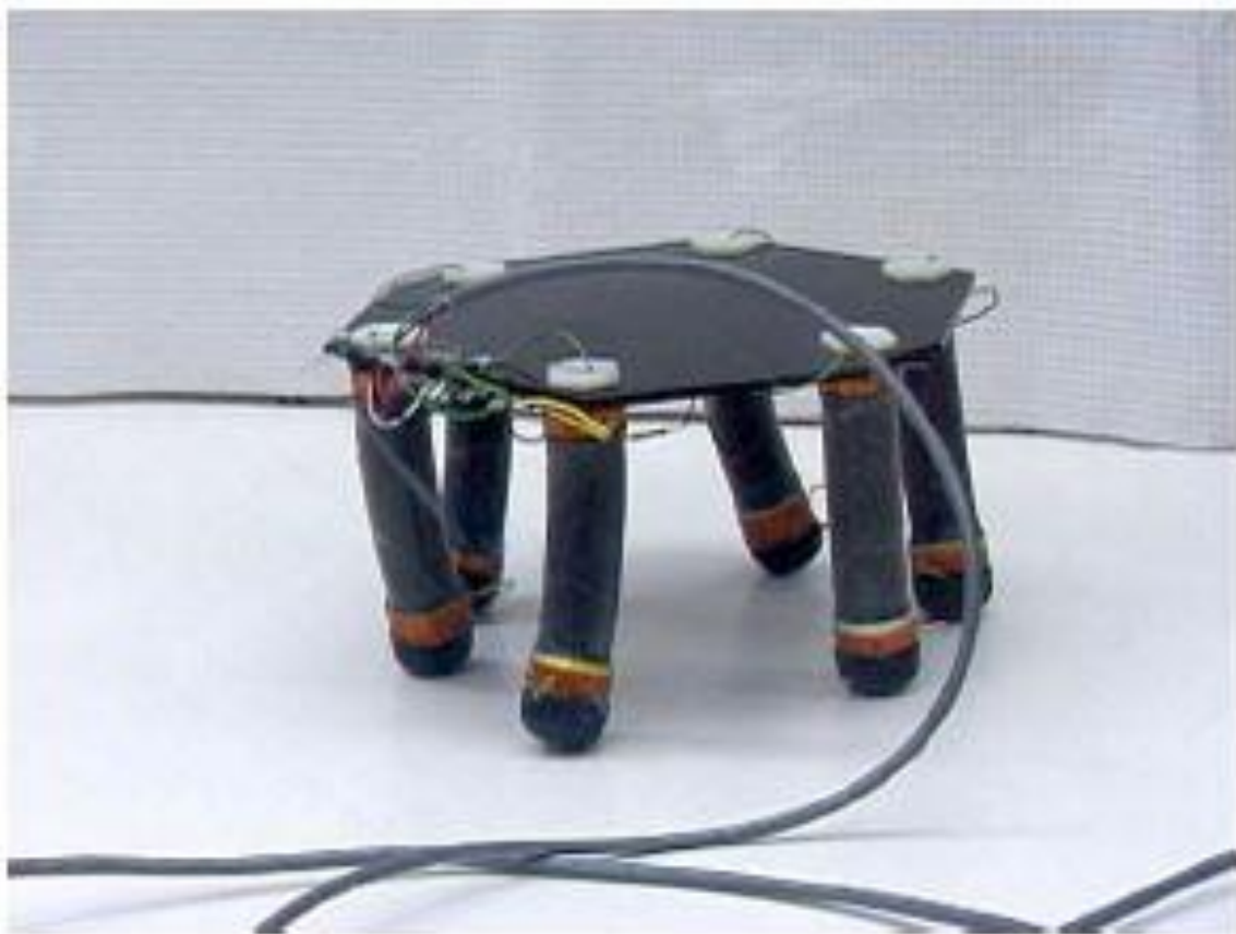
Figure 21. Six-2-DOF-legged soft robot [8]
