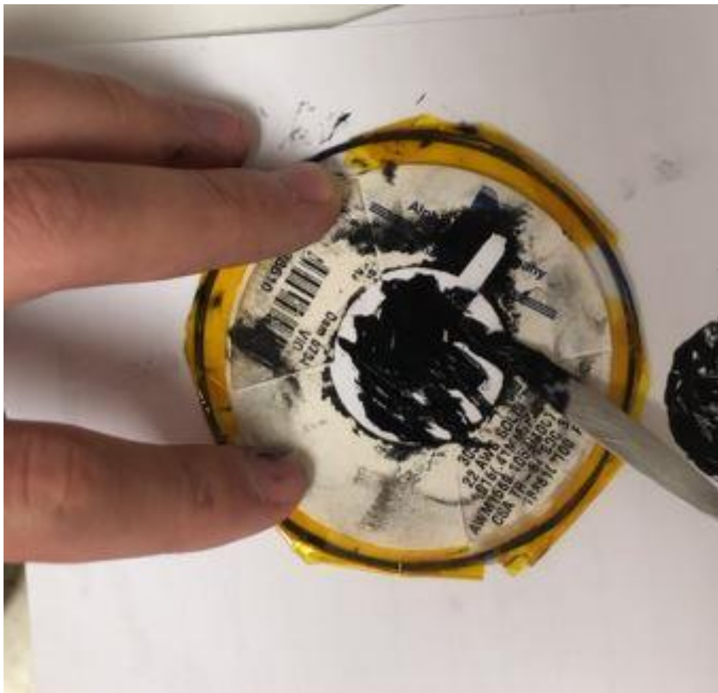
Figure 47. Compliant electrodes spreading
