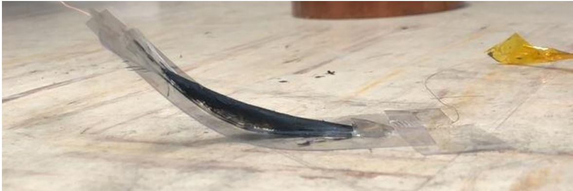
Figure 58. Bending actuator voltage off
