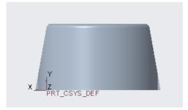
Figure 14: Inclined walls used for the water tank
