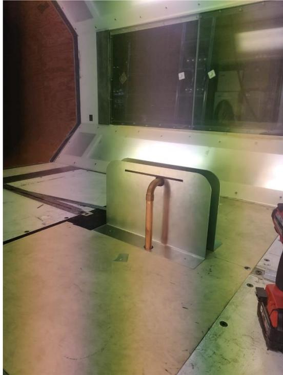
Figure 6.6. Flat plate and aluminum supports screwed to the floor.
