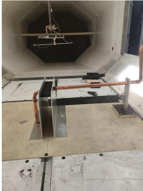
Figure 6.8. experiment structure with both copper tubes connected.
