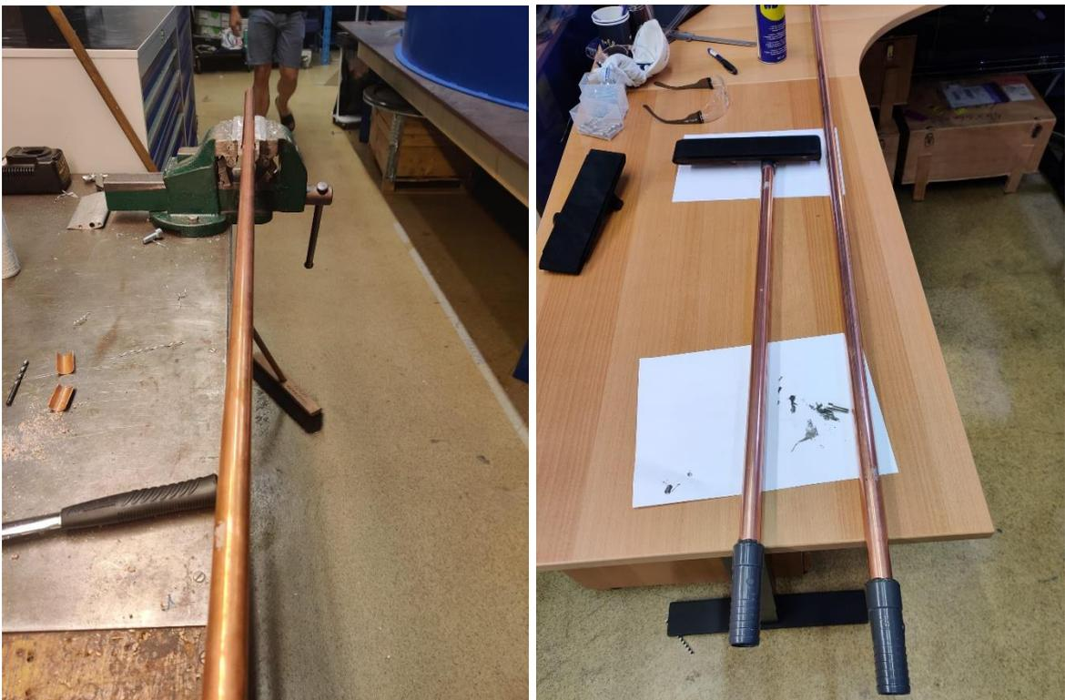
Figure 6.4. Original copper tubes Left. sanded joined tubes with plastic couplings and flat plate Right.
