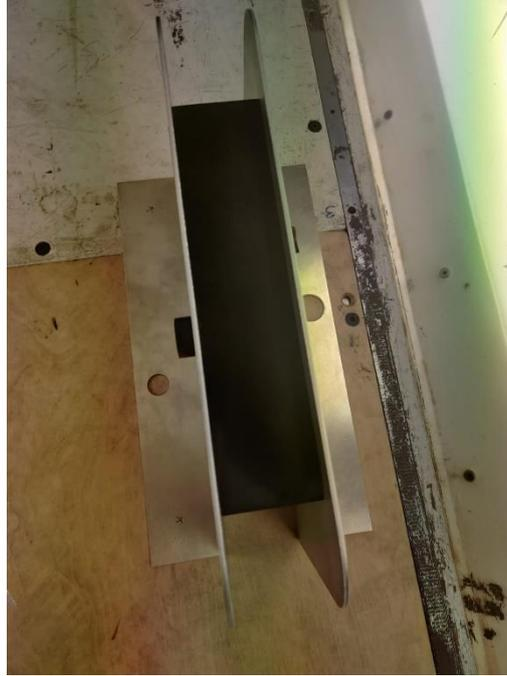
Figure 6.5. Flat plate and aluminum supports joined.
