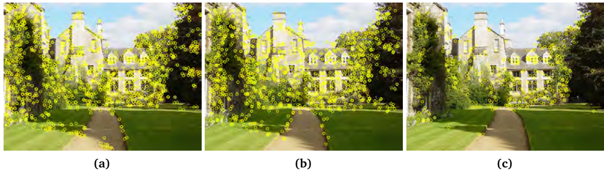
Figure 2.5. Sample SIFT (a), SURF (b), and Star (c) keypoints extracted from an image of the Oxford buildings dataset [Phi+07]. The features were obtained using the default parameters for the three algorithms in the OpenCV library [Bra00].
