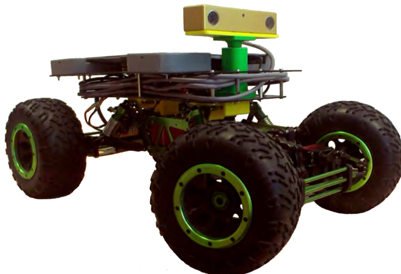
Figure A.4. Robotic platform employed to record the home environment dataset.
