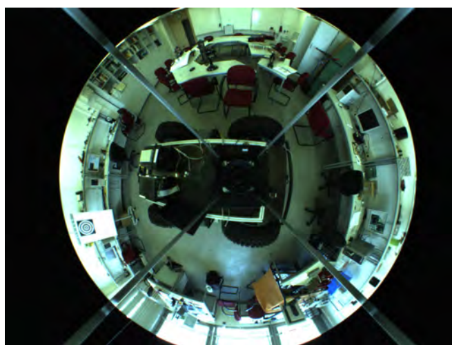
Figure 2.3. Example of an image captured with an omnidirectional camera (© User:Sgeureka / Wikimedia Commons / CC-BY-SA-3.0 / GFDL ).
