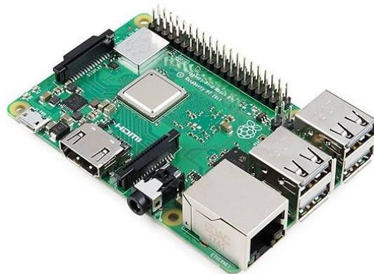
Figura 3.8. Microcontrolador Raspberry Pi 3B+
