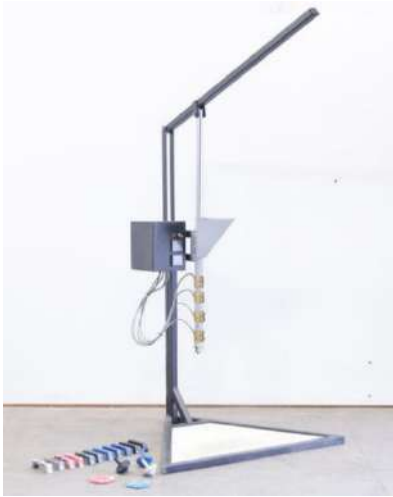
Graph 5: Injection molding machine and table of technical characteristics.
