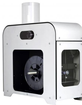
Figura 21. Extrusora 3Devo Composer 350 [37]
