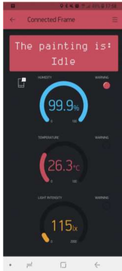
Image 11. App screen when humidity alarm is triggered
