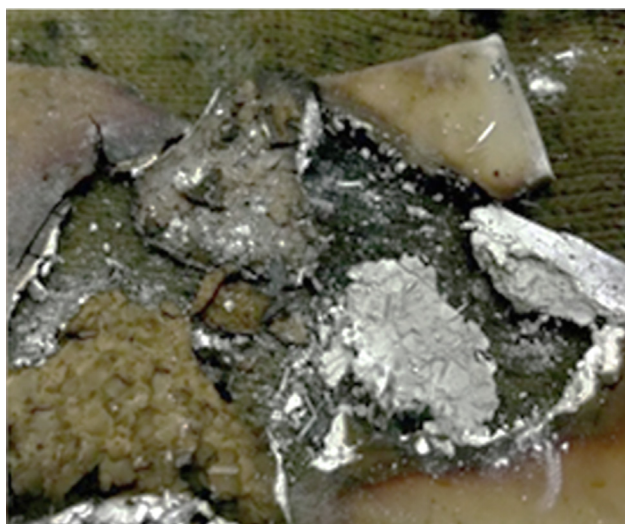
Fig. 12 – Macrograph of carbonized wastes of UPE after fire test of any sample (Picture after a fire test for 30 min of +50M + 3GF bio-composite).
